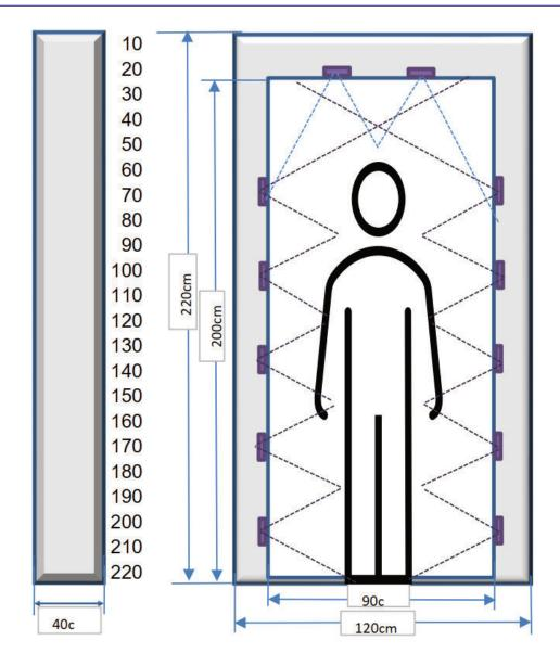
Because the dose of 222nm ultraviolet radiation required to kill more than 99% of the virus is 3 millijoules, people can pass through the disinfection door in 7 seconds to inactivate the virus on the surface of the body.
